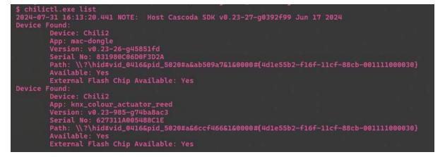
3. Flash the application binary knx\_colour\_actuator\_reed.bin using chilictl.exe. Use the command shown in the picture below. The number that comes after -s should be the serial number that you have identified in the previous step.
