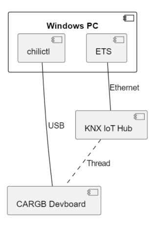
The Demo consists of controlling the CARGB using the Group Monitor on ETS. In order to do this, you will need the following:
