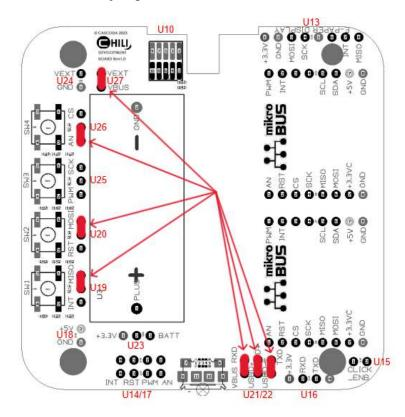
2. Place the RELAY Click, as shown in the pictures at the front page of this document. The end of the RELAY Click which has the relays should face the battery slot. You can insert the Click board on the right or left slot, both are the same.
