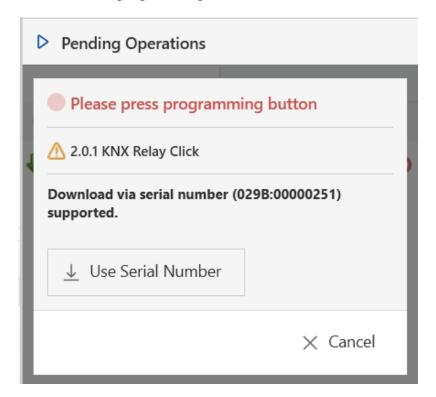
The download by serial number does not require any interaction with the device. All you have to do is click on the "Use Serial Number" button.
