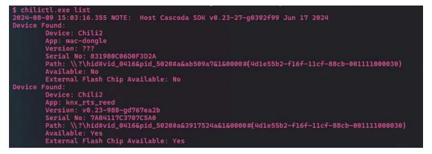
3. Flash the application binary knx\_rts\_reed.bin using chilictl.exe. Use the command shown in the picture below. The number that comes after -s should be the serial number that you have identified in the previous step.
