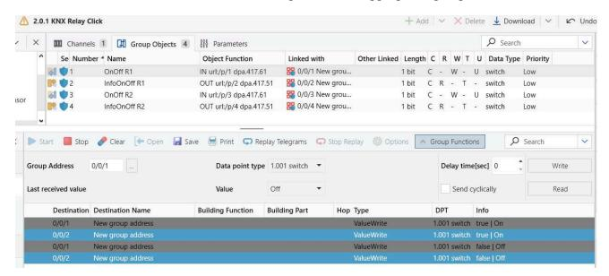
3. To switch RELAY2 of the Relay device ON, select the Group Address linked with the "OnOff R2" Group object, and the same thing as the previous step applies.
